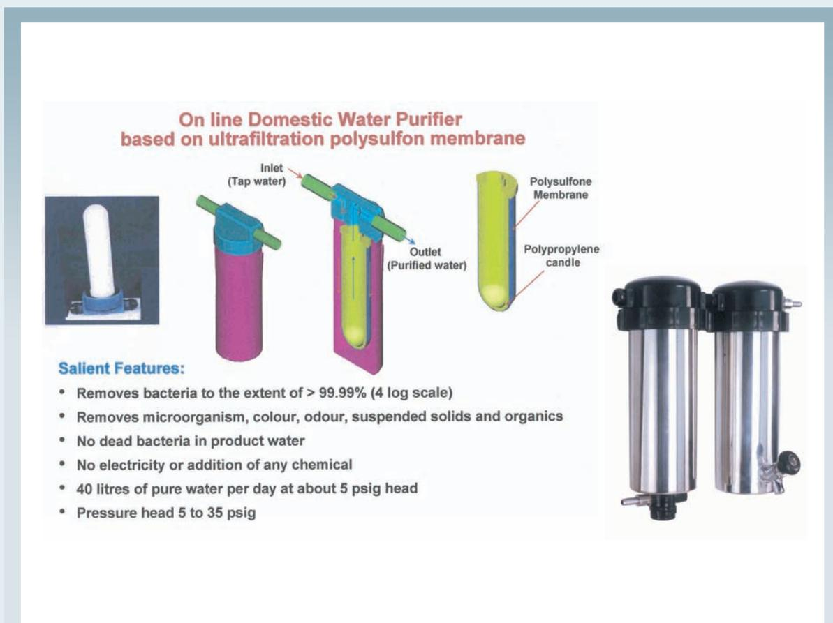
*Water Purifier Developed by BARC*
