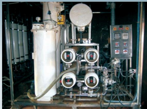
Barge Mounted Desalination plant (50 KLD capacity)
