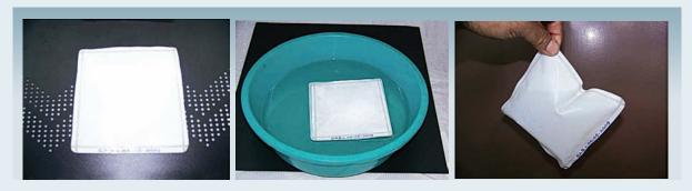
Water purification through Membrane Pouches
