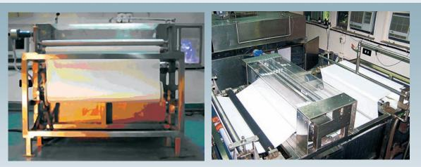
Membrane Casting Machine at BARC
